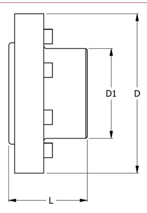
D = 225 D1 = 150 L = 100 Max bore = 90 Torque (N m) = 2000
